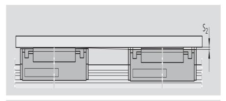
$$S_2 = b \cdot 7 \cdot 10^{-5} \\ S_2 = \text{permissible vertical offset} \\ b = \text{distance between} \\ \text{runner blocks} \\ \text{[mm]}$$
