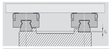
$$S_1 = \text{permissible vertical offset} \qquad [mm] \\ a = \text{distance between guide rails} \qquad [mm] \\ Y = \text{design factor}$$
