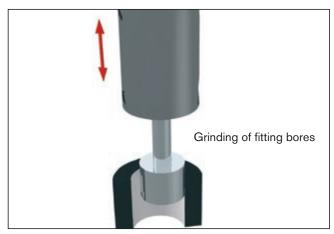
Internal cylindrical grinding
