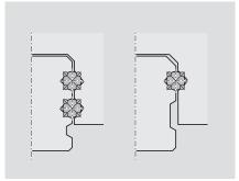
Other ball rail systems with 2 or 4 ball circuits with **4-point contact** have multiple friction: in the Gothic-arch raceway profile, the differential slip at side loading, as well as with comparable preload without load, causes higher friction (depending on the conformity and load, this may be up to approx. 5 times the frictional value).
