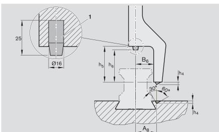
1) Example: Use rubber buffers as contact points while pressing the guide rail in. Material: PUR
